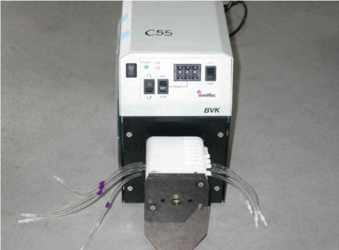
Figure 12 Dosing pump ISMATEC BVK
