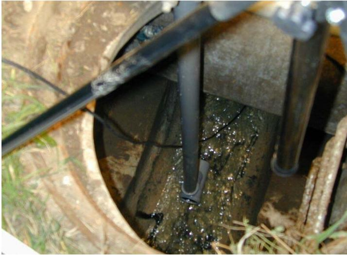
**Figure 7 Dosing tubes holder**
