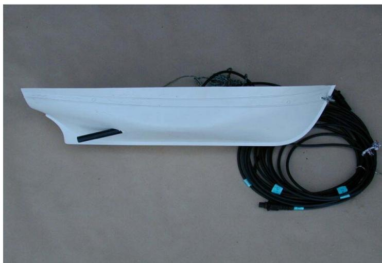
**Figure 6 Boat for the conductivity probes**
