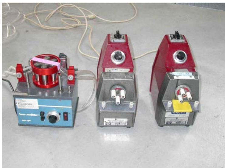
Figure 11 Peristaltic sampling pumps
