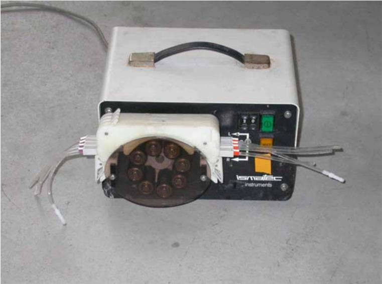
Figure 13 Dosing pump ISMATEC MV-CA4
