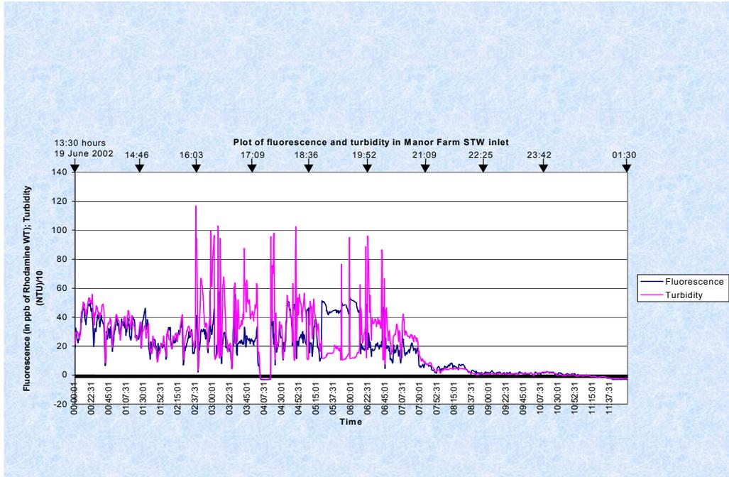
**Figure 4. Temporal variation in fluorescence and turbidity monitored in raw sewage entering Manor Farm STW, Reading**
