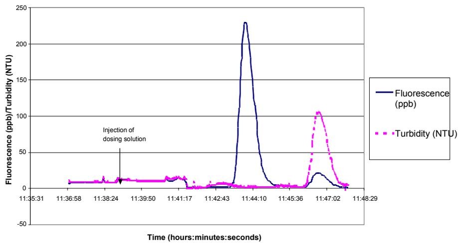
**Figure 2. Downstream sewer monitoring of fluorescence and turbidity after dosing with 20ml of 200 mg/l of Rhodamine WT**
