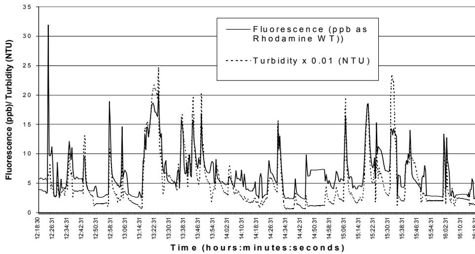
**Figure 1. Temporal variation in fluorescence and turbidity within a small foul sewer.**
