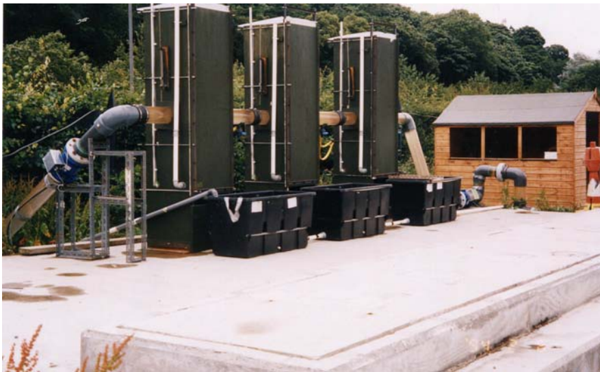
Figure 1. Overall view of the test rig showing the pipe passing through the test boxes.
