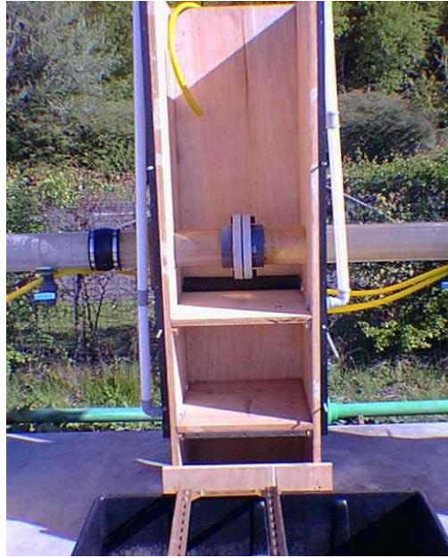
Figure 3. Internal construction of a test box showing the location of the pipe defect.
