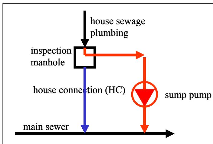
**Figure 1:** *Elimination of the inflow of domestic water from house sewage plumbing*
