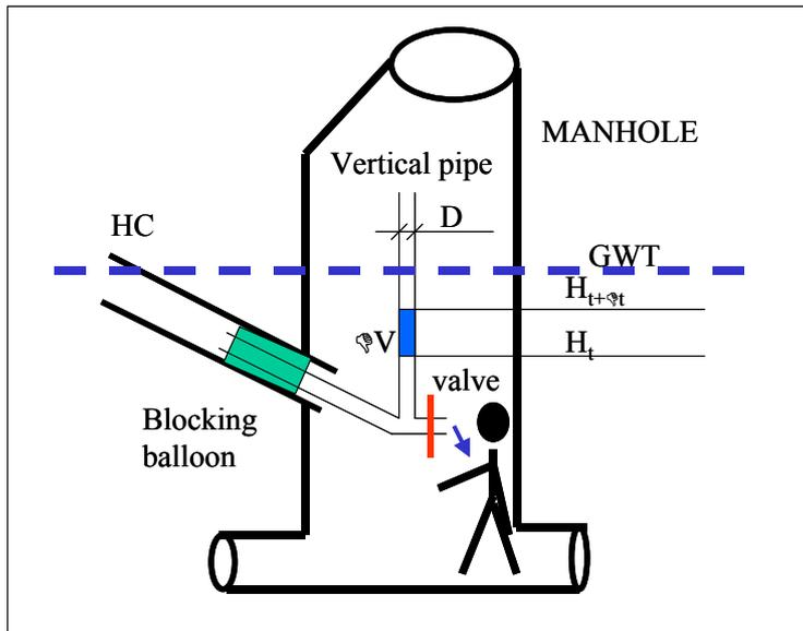
**Figure 4:** Scheme of installation of a blocking balloon and a vertical pipe in a manhole
