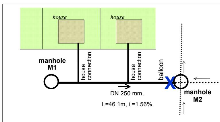
**Figure 2 :** Layout of the experimental site. Measurement of the two HC pipes and connecting sewer (Prague-Troja catchment)
