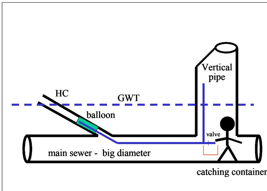
**Figure 8:** *Scheme of installation of the measurement equipment in a house connection connected to passable sewer*
