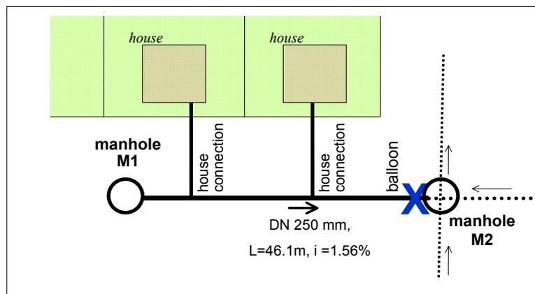
**Figure 4:** Measurement of two HC pipes and connecting sewer in Praha-Troja catchment (sealing balloon- marked with blue cross)
