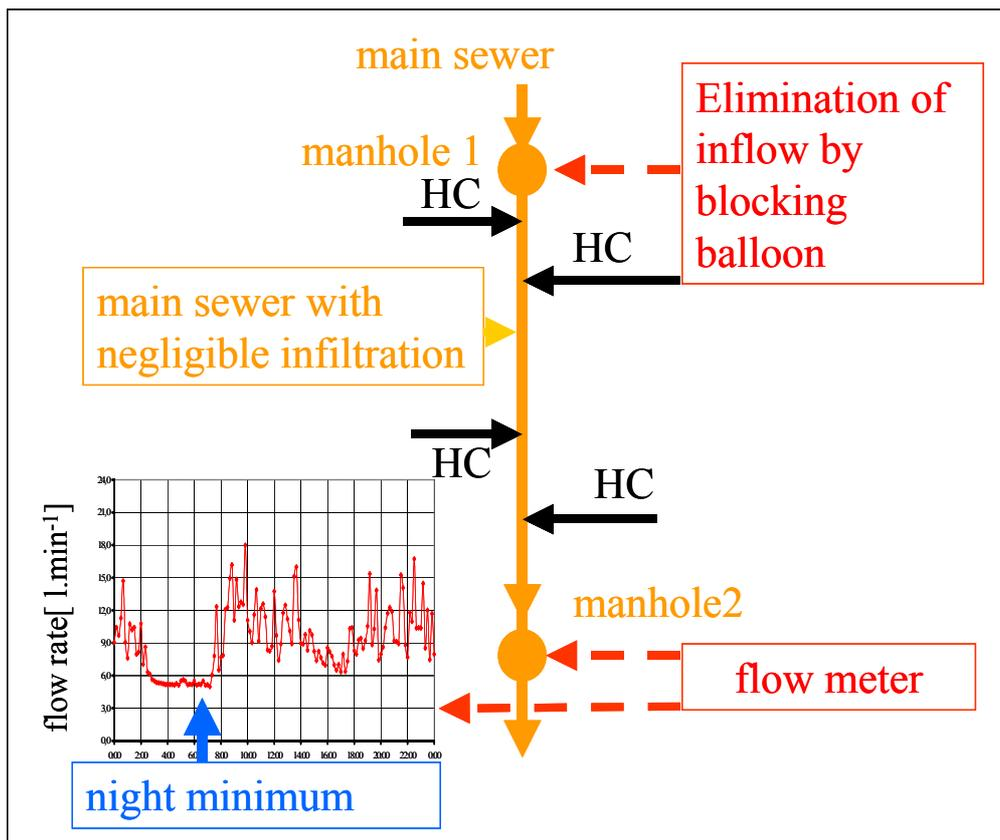
**Figure 11:** Scheme of installation of the measurement equipment in small reference catchment
