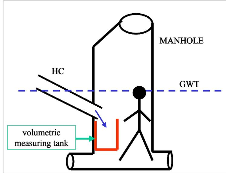
**Figure 3:** Scheme of installation of the measuring volumetric tank in a manhole
