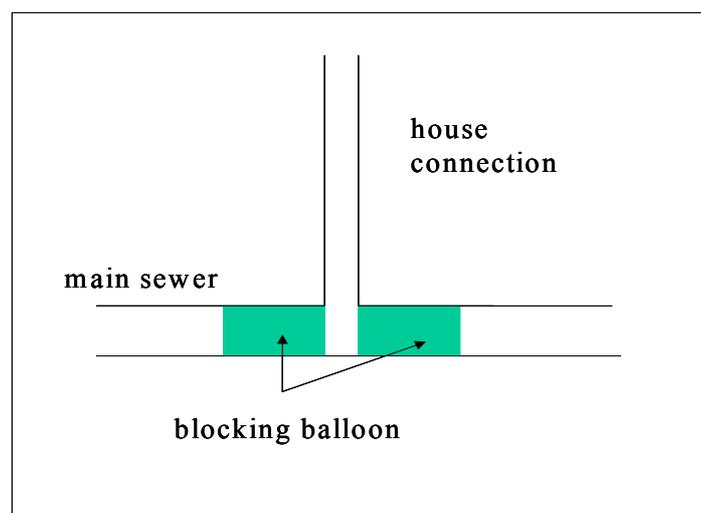
**Figure 10:** *Blocking of house connection using two balloons in main sewer*
