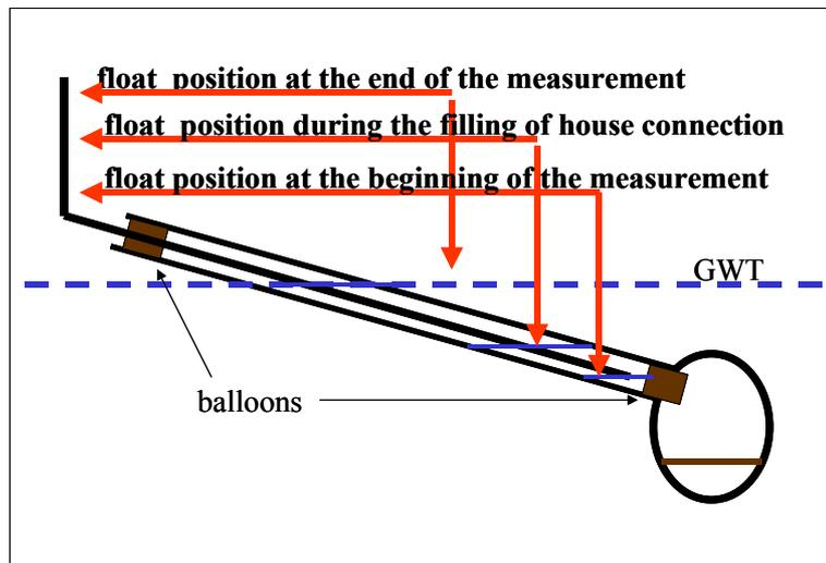
**Figure 9:** *Scheme of installation of the measurement equipment in case of a non-passable sewer*
