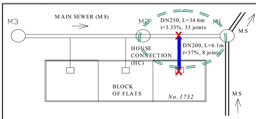
**Figure 1** : Sample map documentation (thick blue line – tested segment, crosses – sealing balloons, dashed line – examined section)
