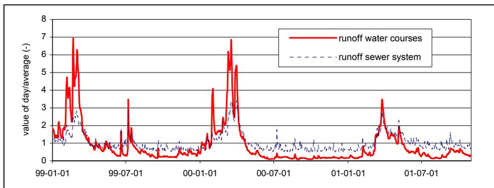
Figure 12: Normalised flow rate measurements of water courses and sewer system in the City of Dresden
