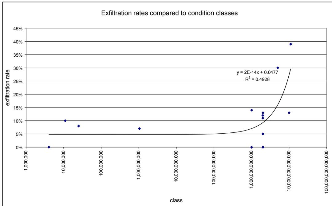
Figure 21: Comparison of exfiltration rate and condition of sewers
