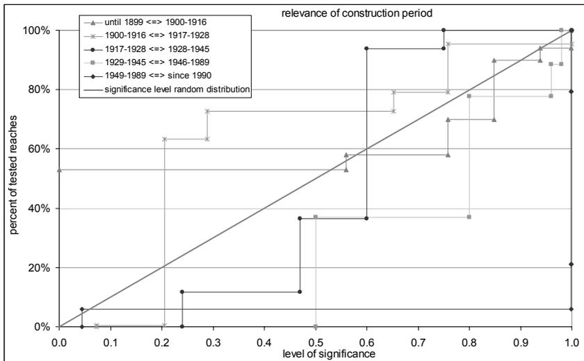
Figure 10: Relevance of construction period for condition classes
