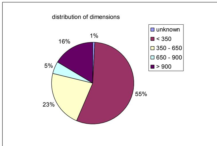
Figure 15: Distribution of diameters in the sewerage system of Dresden
