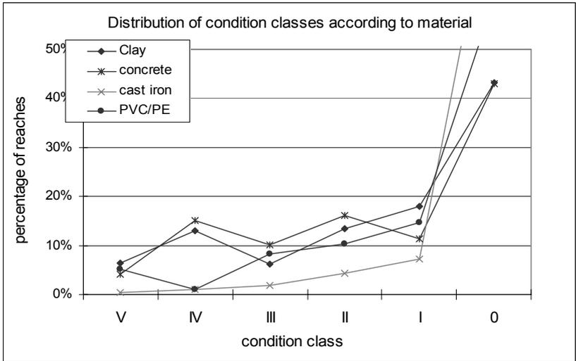
Figure 6: Distribution of condition class with respect to material
