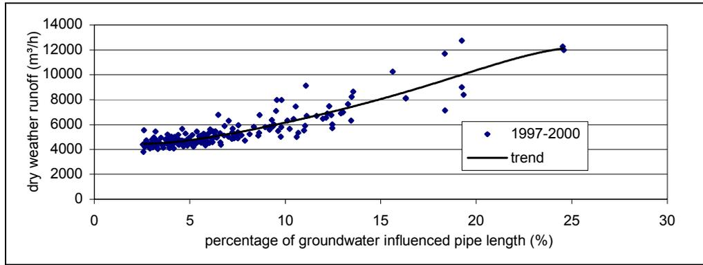
Figure 13: Correlation between percentage of groundwater-influenced length of sewer pipes and dry-weather runoff
