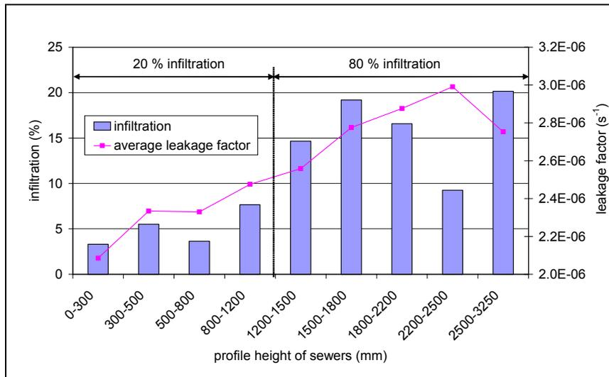
Figure 14: Infiltration and leakage factors depending on the profile height of sewers in the City of Dresden
