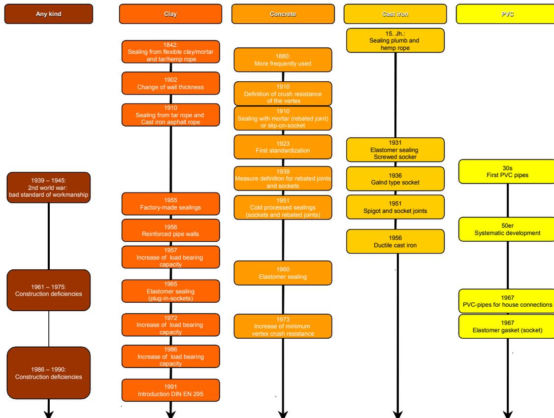
Figure 2: Development of the sewer construction [derived from Stein and Niederehe, 1992]
