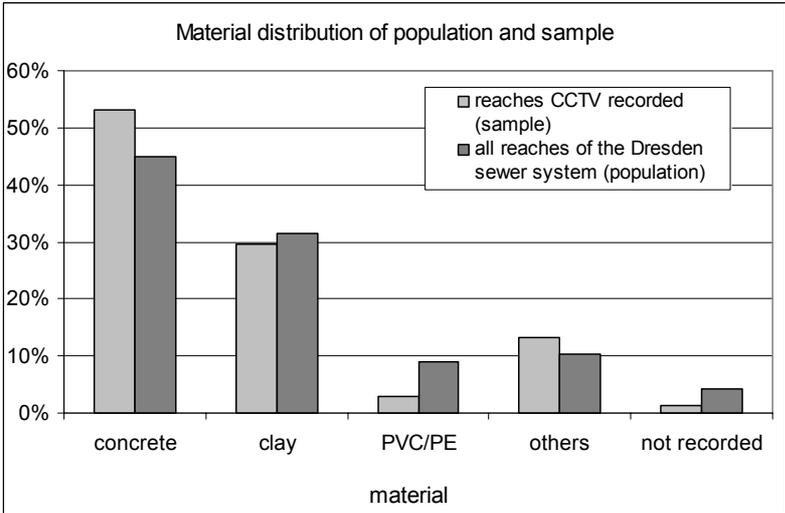
Figure 3: Comparison of the dataset of the whole sewer system and the sample (Material distribution)
