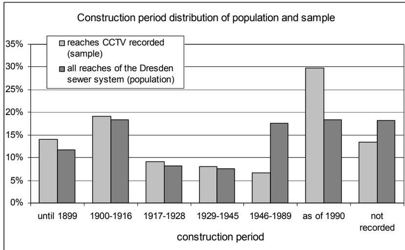
Figure 5: Comparison of the dataset of the whole sewer system and the sample (construction period distribution)
