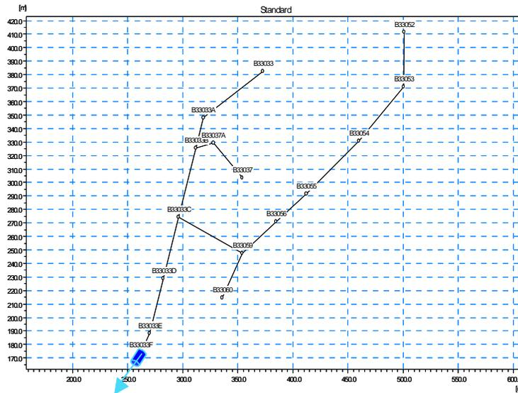
Figure 8 – Borel sewer system
