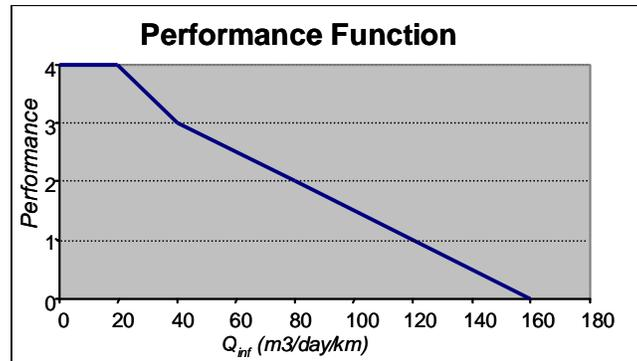
Figure 10 – Performance function for infiltration flow
