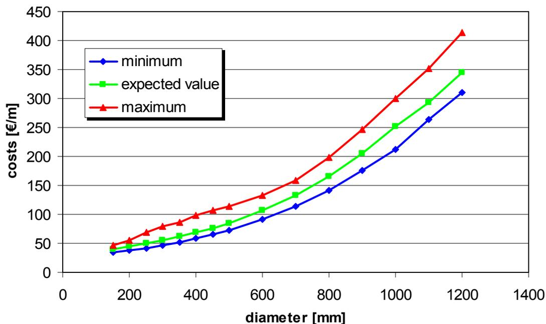
Figure 5-1: Costs for sewer pipe including delivery, installation and testing of leaks (all earthworks like ground evacuation etc. are not included)
