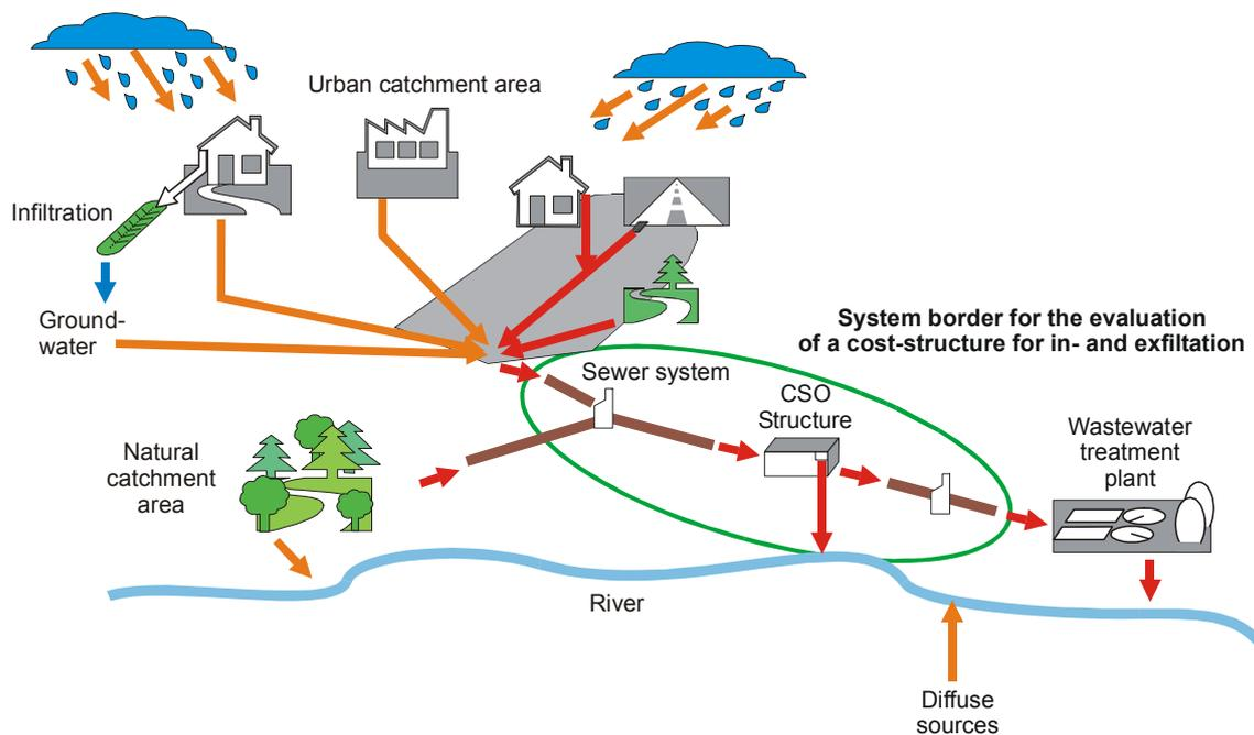
Figure 2-1: System border for the evaluation of cost-structure for in- and exfiltration
