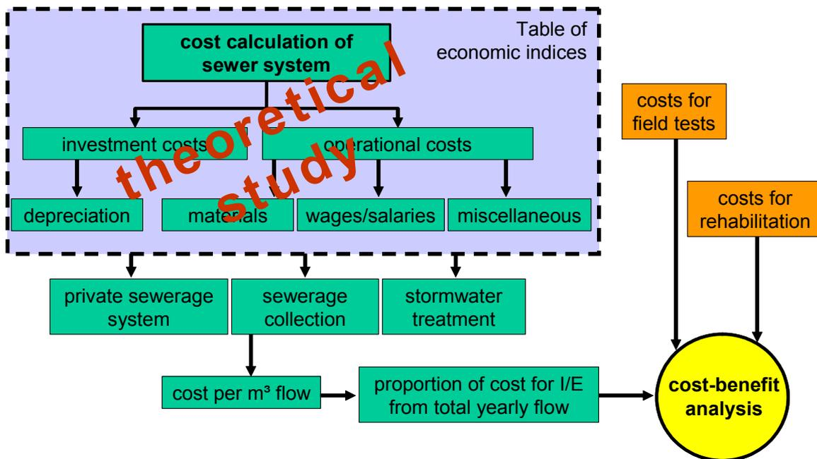
Figure 4-3: Procedure for the cost-benefit analysis
