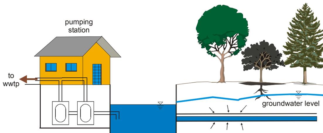
Figure 2-4: Simple example of a pumping station and increasing costs aroused by infiltration
