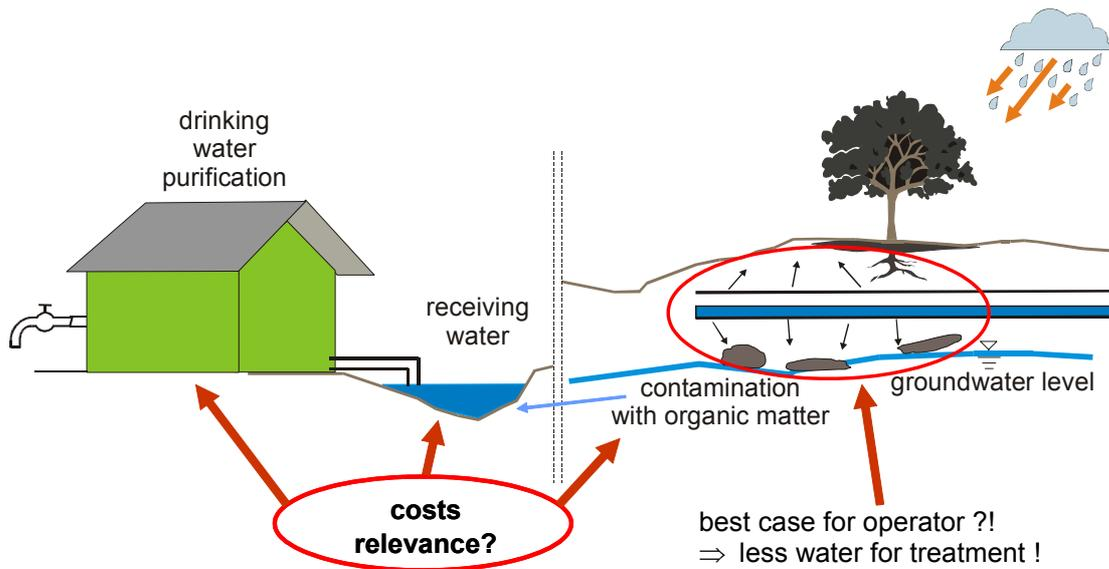
Figure 2-5: Example for exfiltration and apparently decreasing costs for operation
