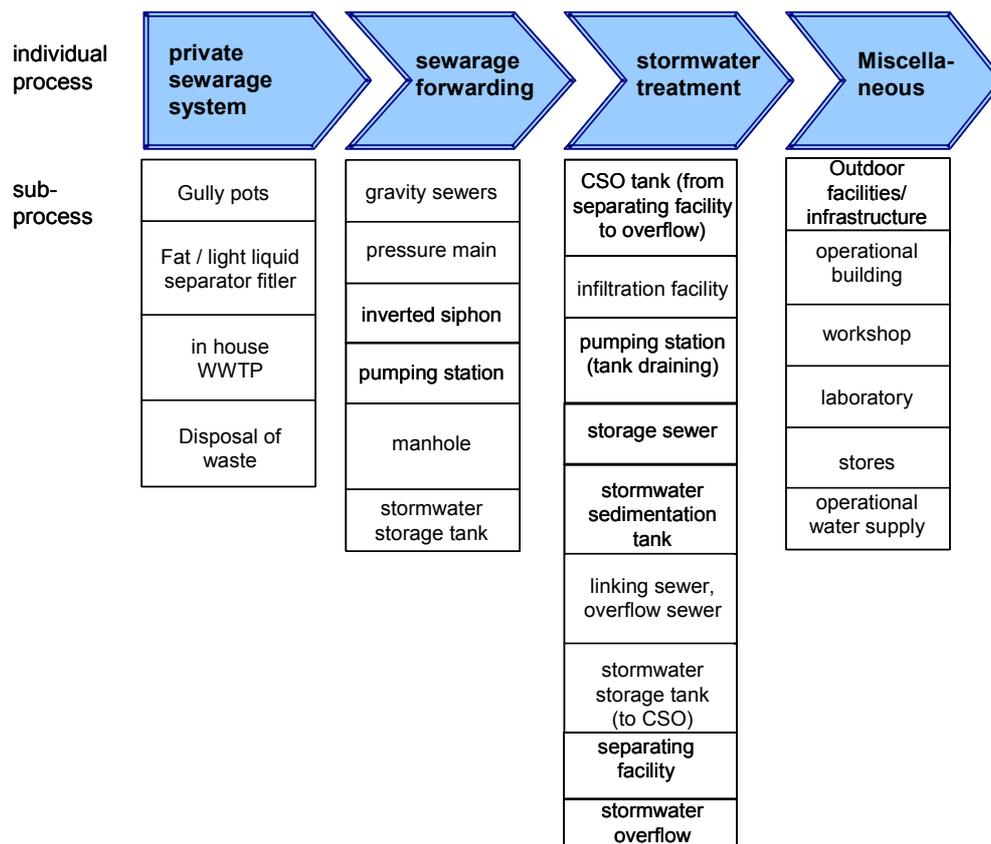
Figure 2-2: Process model of a sewer system (modified from EG/LV, 2003)
