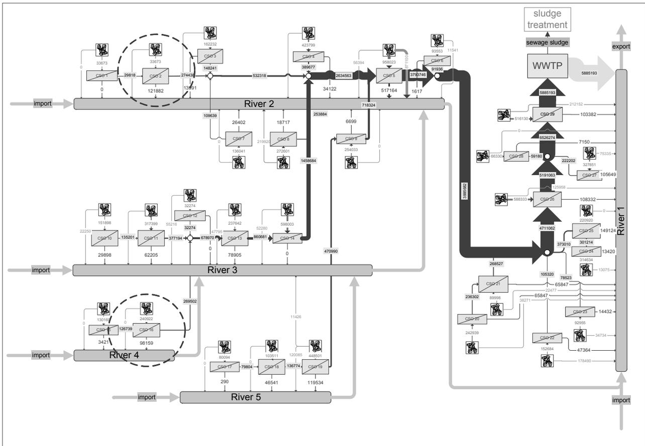
Figure 7 – Substance flow: water (in  $m^3/y$ ) for the wastewater system in catchment I.
