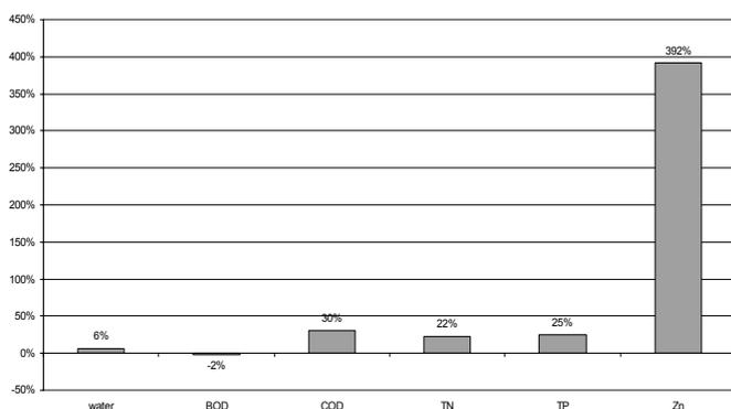
Figure 2 – Gaps in the sewer mass balances; outputs minus inputs.
