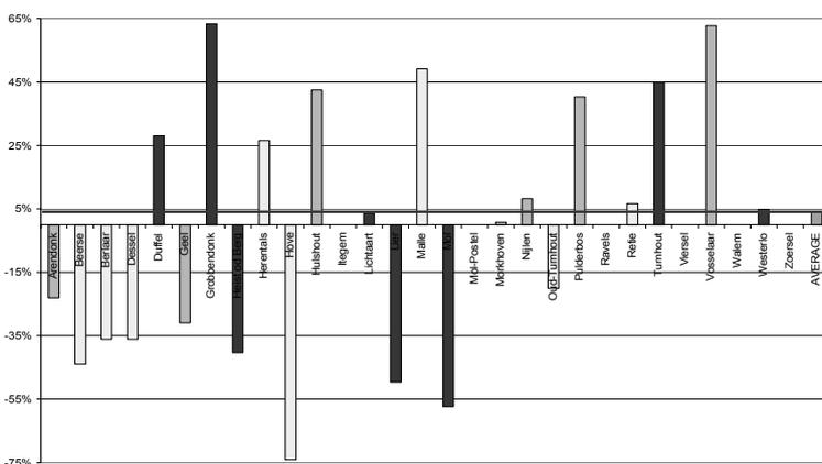
Figure 4 – Percentages of estimated CSOs (relative to the total stormwater entering the sewer) for the 29 Nete catchments; in medium grey are reliable data, in light grey less reliable data, in dark grey scarcely reliable data.
