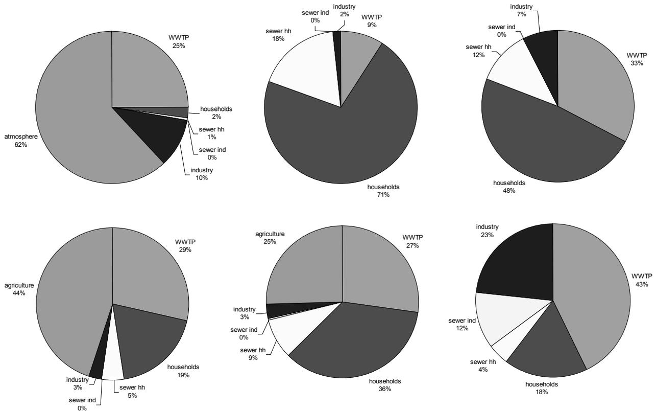
Figure 3 – Relative loads into the Nete river – from left to right and from up to down: water, BOD, COD, TN, TP and Zn; “sewer ind” and “sewer hh” indicate the loads discharged in the receiving water via the sewer network by industry and household respectively.
