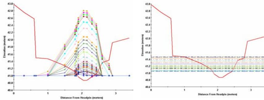
figure 4 - PHABSIM – results of flow velocities and depths calibration
