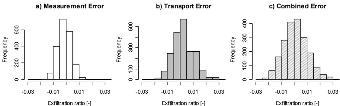
**Figure 4 a) Error estimation from the measurement uncertainty; b) Estimated error contribution from the dynamic behavior of the system c) Combined uncertainty of both error contributions to the exfiltration ratio**
