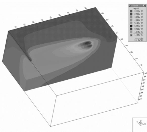
Fig. 4: 3-dimensional modelling of a single leaking sewer in Rastatt.
