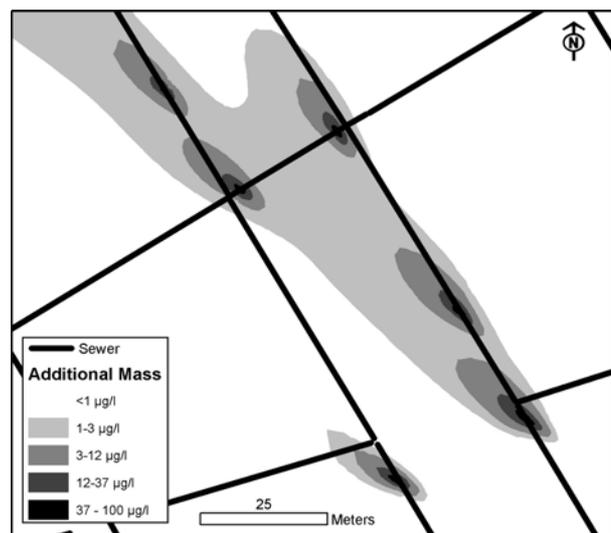
Fig. 5: Implementing sewer leaks as point sources into numerical groundwater models.
