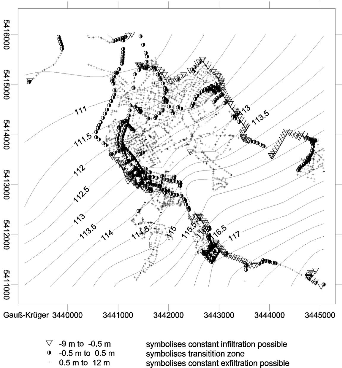
Fig. 3: Position of sewers in Rastatt in relation to groundwater level (m.a.m.s.l. measured at 7.9.2001).
