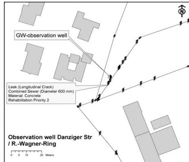
Fig. 2: Detail from the sewer defect database used for site selection. Thunderbolts indicate cracks in the sewer.
