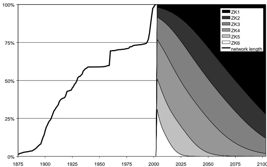
**Figure 5:** Condition forecast for the inspected sample of sewer pipes
