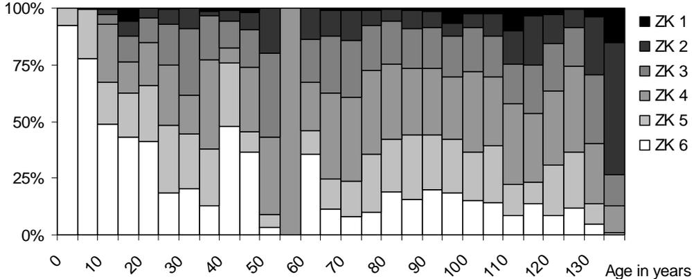
**Figure 1:** Distribution of condition grades (ZK), relative length
