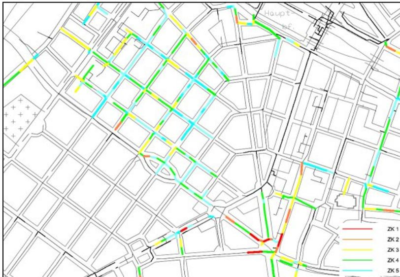
**Figure 6:** Priority map of an inspected sewer network
