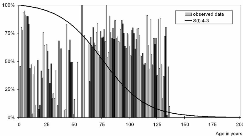
**Figure 3:** Calibrated transition function from condition state 4 to 3
