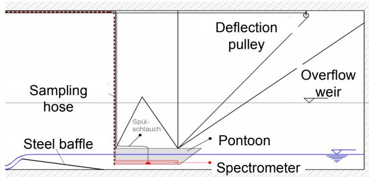
Figure 1: Installation of a submersible spectrometer in a pontoon for continuous measurements in a CSO-chamber
