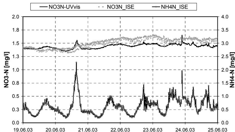
Figure 7: Ammonium and nitrate concentrations in the Danube river downstream the main Vienna WWTP. ISE=Ion-sensitive sensor; UVvis=UV-VIS-spectrometer
