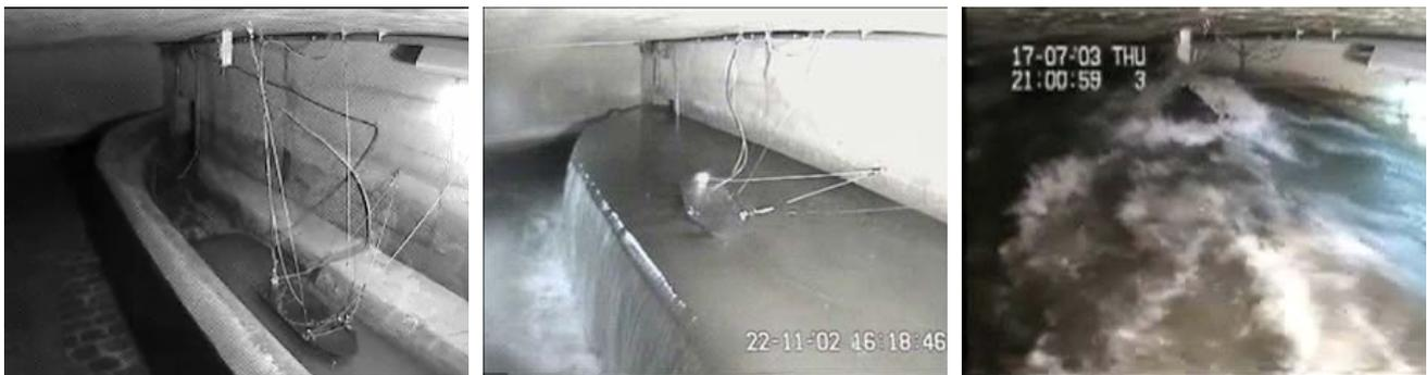
Figure 2: Floating pontoon with spectrometer under varying flow conditions. Left: Dry weather flow, Middle: CSO overflow, Right: Extremely high flow
