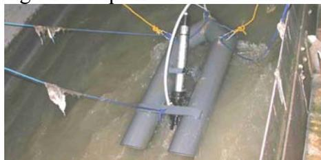
Figure 3: Installation of an ISE-ammonium probe in an open sewer channel
