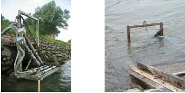
Figure 4: Compact water quality monitoring station at the Danube near Vienna. Left: Water level too low (probes dry). Right: Submersion depth approx. 1 m
