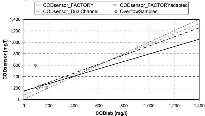
FACTORY=factory calibration; FACTORYadapted=linear regression of factory calibration based on reference measurements; DualChannel= linear regression function (Abs(254 nm)-Abs(436 nm))
