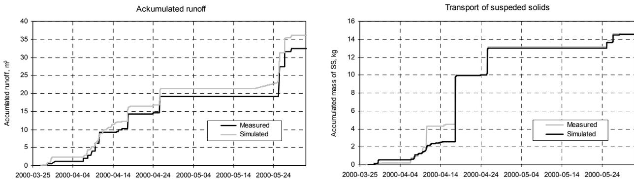
**Figure 9 and 10** Measured and modelled accumulated road runoff (m<sup>3</sup>) and load of SS (kg).
