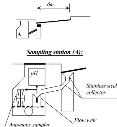
**Figure 2 and 3** The road side at Södra Hamnleden in Luleå and a plan view of approximate catchment area (broken lines) and a section view of the sampling station.
