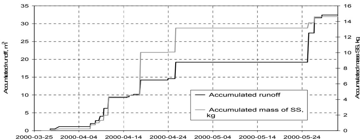
Figure 4 Accumulated runoff ( $m^3$ ) and massload of suspended solids (kg) during the measuring period.
