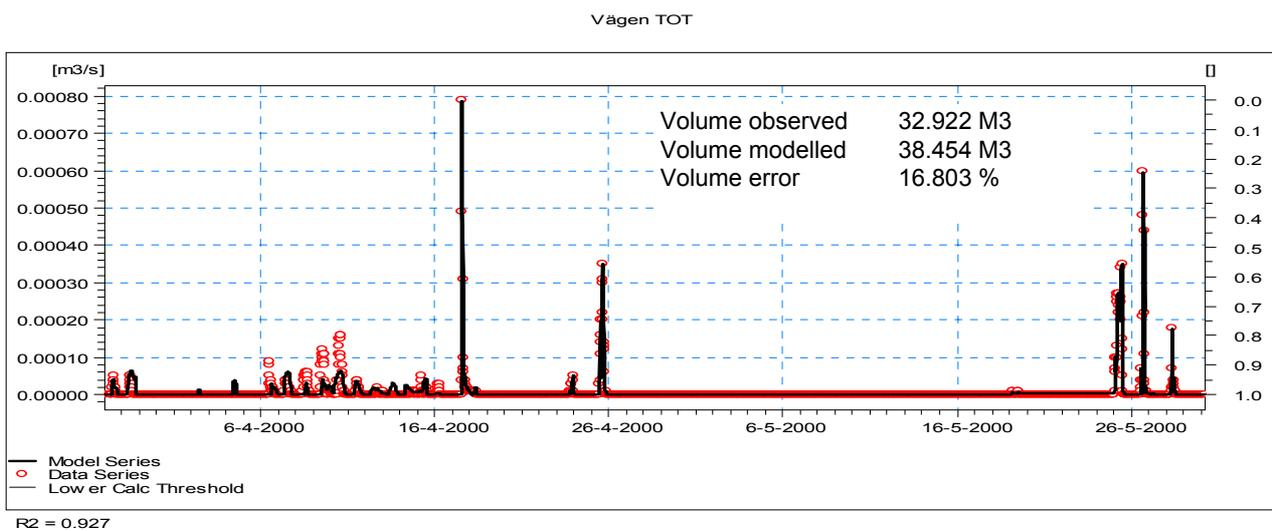
Figure 7 Measured and modelled volume of road runoff during the measuring period.
