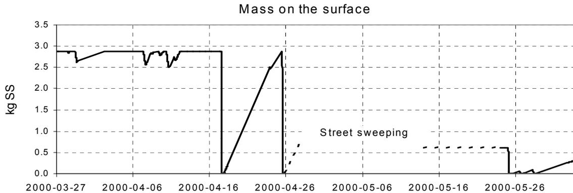
**Figure 8** Mass of SS (kg) on the surface of the catchment area.
