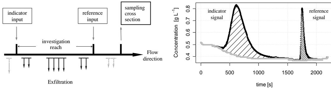
**Figure 1** Left: Conceptual sketch of the experimental set-up of the QUEST method. Right: Example results of a QUEST experiment showing the concentration time series of an arbitrary tracer at the sampling cross section. Both figures taken from (Rieckermann et al. 2005b).
