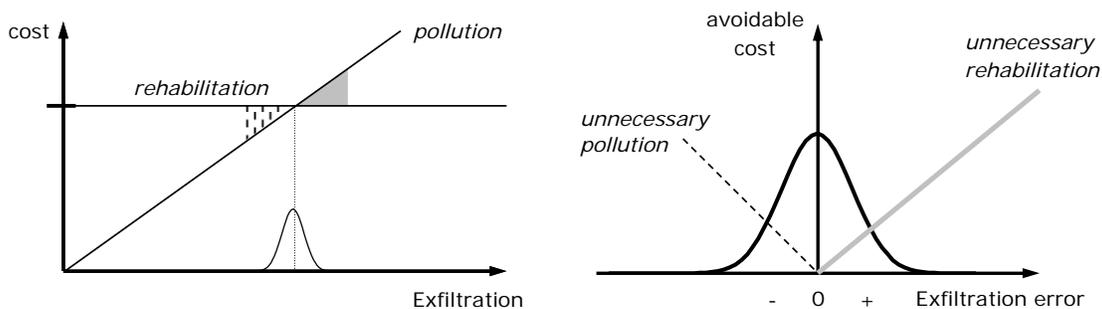
**Figure 3. Left: Simplified cost functions for sewer rehabilitation (adapted from Reckhow (1994)). Right: The marginal increase in costs associated with uncertainty in the tracer method. Layouts that have a low measurement error would have lower expected cost.**
