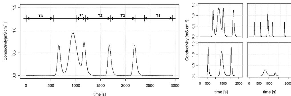
**Figure 2.** Left: Timing-parameters of a QUEST experiment: T<sub>1</sub>=time between indicator and first reference pulse, T<sub>2</sub>=time between reference pulses, T<sub>3</sub>=time outside peak span that is used for data analysis. Right: Examples of possible experiments indicating different combinations of T<sub>1</sub>, T<sub>2</sub>, T<sub>3</sub> and N<sub>R</sub>, M<sub>R</sub>, M<sub>I</sub>.
