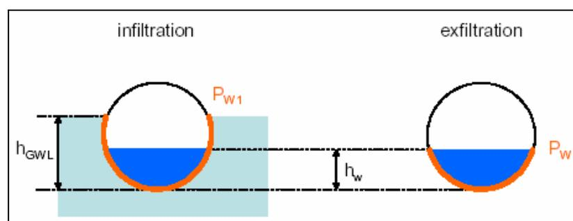
**Figure 2.** Key state variables used in the I/E models.
