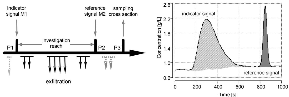
**Figure 1.** Principle of exfiltration measurement (adapted from Rieckermann and Gujer, 2002)
