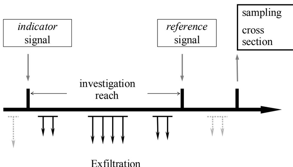
**Figure 1** Conceptual sketch of the experimental set-up of the QUEST method
