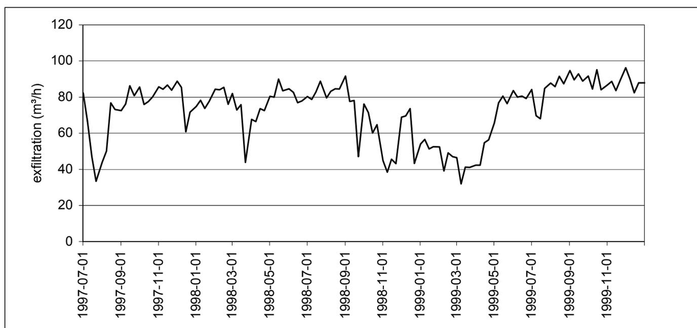
**Figure 1 Simulated exfiltration rates from 1997 to 1999 in a catchment of Dresden**
