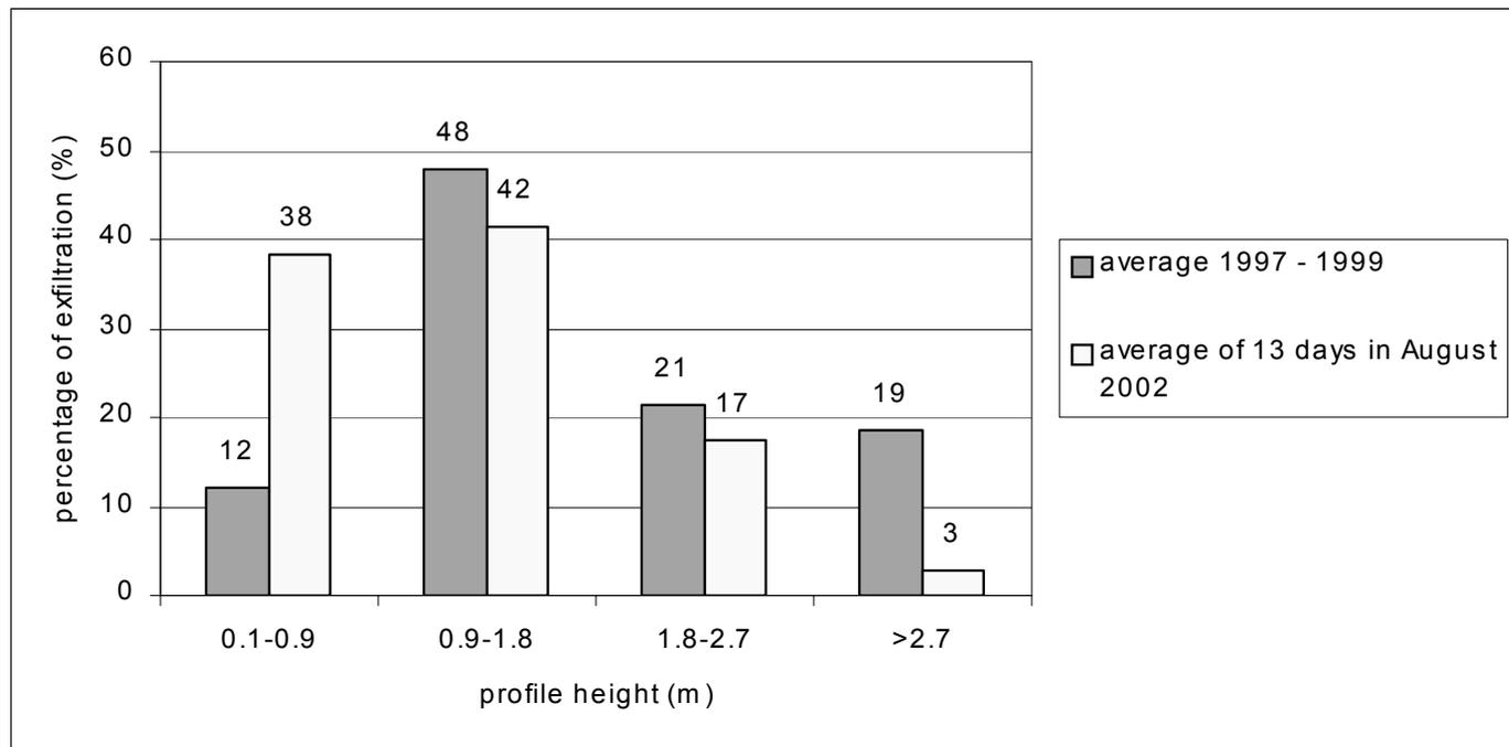
**Figure 3** Percentage of exfiltration from 1997 to 1999 and during the flood event 2002 classified by the profile height of pipes
