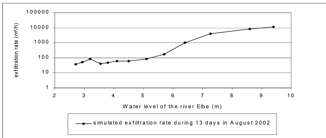
**Figure 2 Exfiltration rates during 13 days of the flood event in August 2002 in dependence on the water level of the river Elbe**
