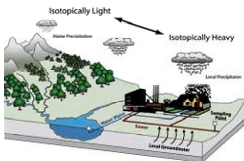
Large-scale meteorological processes are responsible for the varied isotopic signatures of natural waters in different hydrological zones. If the isotopic compositions of drinking water and local groundwater are sufficiently different, they are a suitable tracer to measure infiltration. Such usable isotopic separations can exist, where the drinking water originates from a distant hydrological regime but groundwater is recharged by local precipitation.
