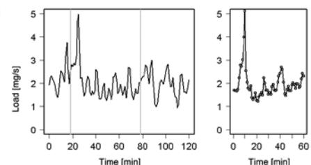
Left diagram: forecasted variations of benzotriazole (silver protection contained in dishwasher detergents) in the sewer. Right diagram: effectively measured benzotriazole loads.
